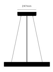
598 mm [ type. **19.0 CASCADE.** ] [ info. MEASUREMENTS.] 60 mm Customisable cable drop up to 10m [ info. **SPECIFICATIONS.**] GU10 / 220-240VAC / IP20 145 mm Max 19 x 9W LED GU10 bulb Bulbs sold separately
