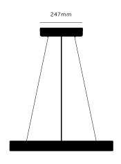
798 mm [ type. **31.0 CASCADE.** ] [ info. MEASUREMENTS.] 60 mm Customisable cable drop up to 10m [ info. **SPECIFICATIONS.**] GU10 / 220-240VAC / IP20 145 mm Max 31 x 9W LED GU10 bulb Bulbs sold separately
